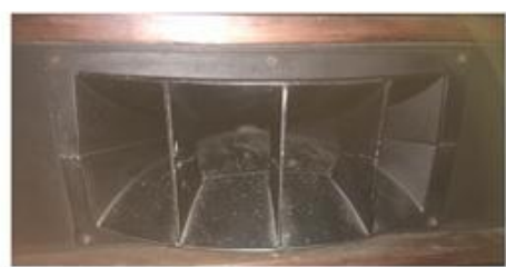
Figure 4 Real Altec Lansing 811B sectoral horn
